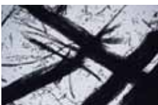
Inferior wood fiber magnified 45 times.
